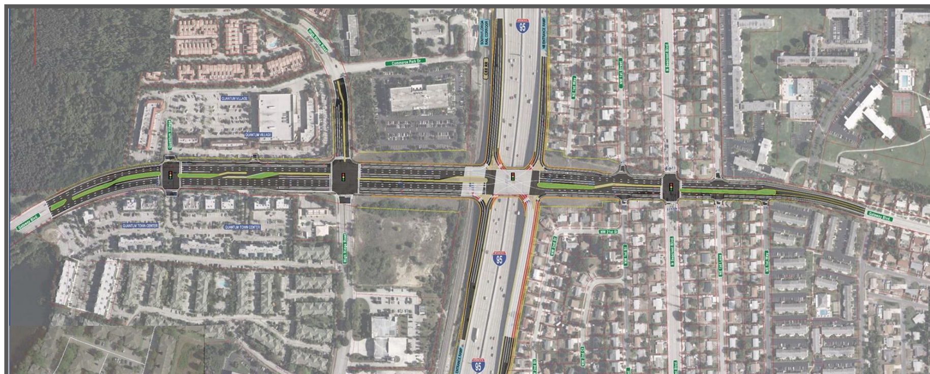
Gateway Boulevard – Single Point Urban Interchange
